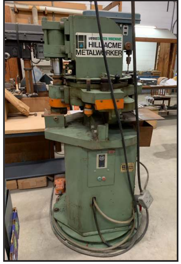
HILL ACME CO MODEL 30 HYDRAULIC IRONWORKER METALWORKER 30 TON CAP PUNCH SHEAR & NOTCH
