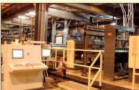
Exit Section, Pinch Roll Stand & Exit Shear: 12" Urethane Rolls, AC Roll Drives, 6" Throat, Hyd. Actuated, 65"W x .080 max. Sheet, Guide Out Table
