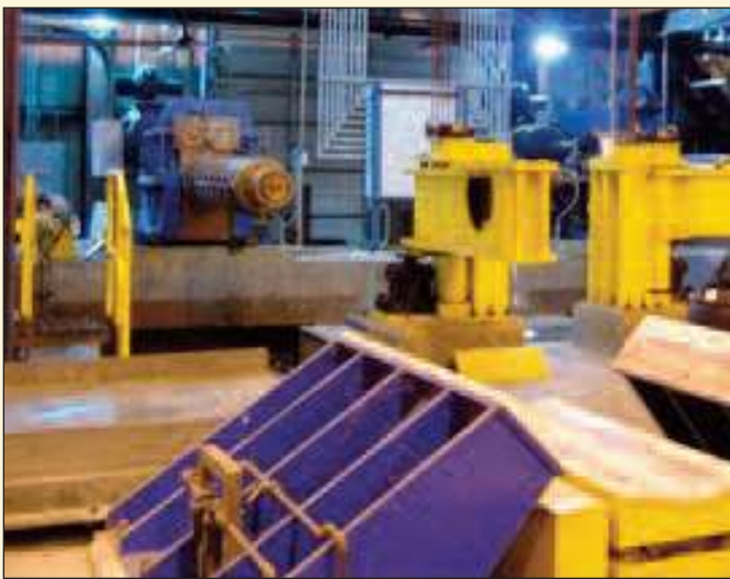
Entry Section, Pay-off Stand: 72" max. Coil size, 20" Mandrel. Outboard Bearing, Hydraulic Feed Roll, +/- 3" Side Set, 12:1 gear ratio, 200 HP AC
