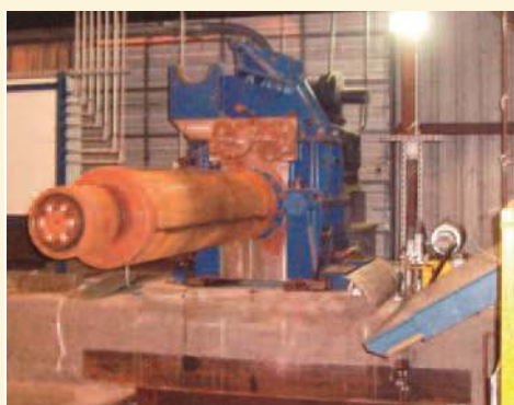
Rewind Stand: 72" max. Coil, 20" Mandrel, Outboard Bearing, Hyd. Feed Roll, 200 HP AC Motor
