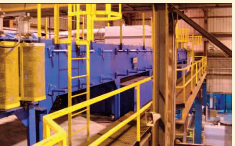
Rinse Section, Hot Water Rinse: (2) 29' Long Sections, 20 Spray Bars, 150 Nozzles, 660 GPM @40 PSI
