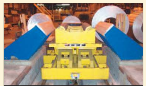
Rewind Coil Car: 30,000 Lbs Southworth, Self Contained Hyd. Unit, Urethane Covered Rollers
